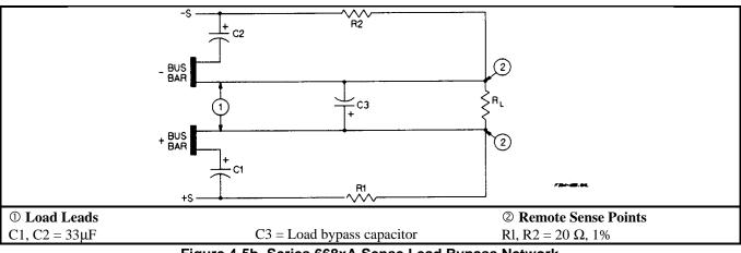
Figure 4-5b. Series 668xA Sense Lead Bypass Network
